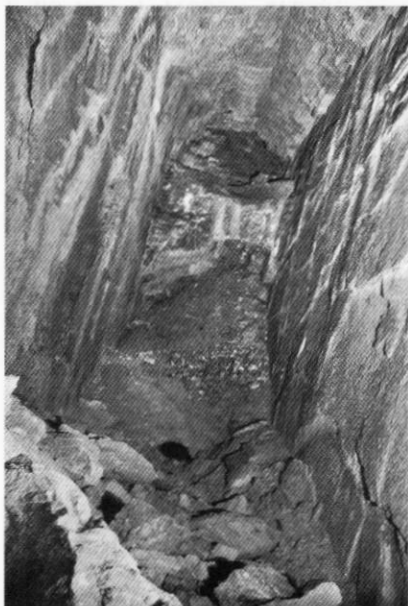
Looking south in the Wrens Nest East with 'Thin Bed' limestone workings. This is the mine destined to be reopened. In this photograph the canal tunnel is behind the camera; there is an upper gallery extending over the canal tunnel. For scale the limestone bed is 28 ft thick and dips at 87° to the east.
